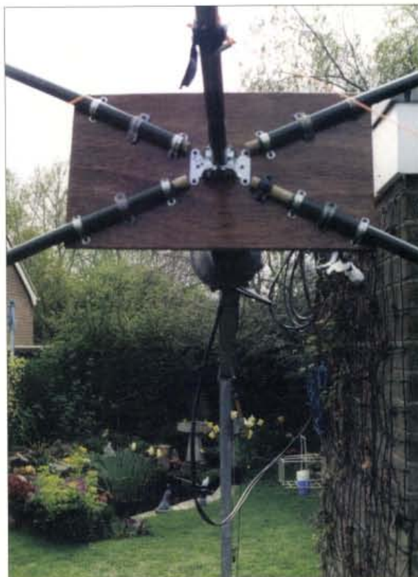
● Fig. 2: Vic's fibreglass (and bamboo) poles fitted to plywood with conduit clamps.
